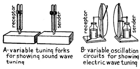
Fig. 36.—Sound Wave and Electric Wave Tuned Senders and Receptors.
