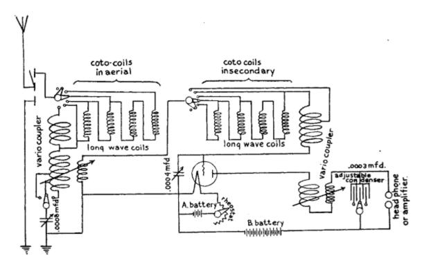
Fig. 59.—Wiring Diagram Showing Long Wave Receptor with Variocouplers and 8 Bank-wound Inductance Coils
