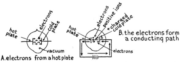
Fig. 70.--Action of Two-electrode Vacuum Tube.
