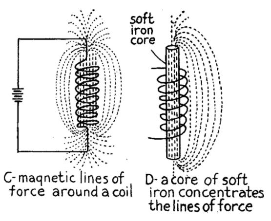
(C) and (D) Fig. 32.—How an Electric Current Sets up a Magnetic Field.
