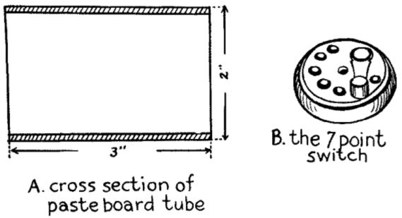
Fig. 97.—How the Tuning Coil is Made.
