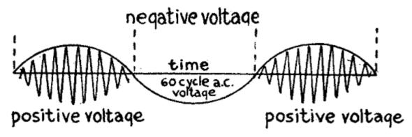
Fig. 95.—Positive Voltage only sets up Oscillations.
