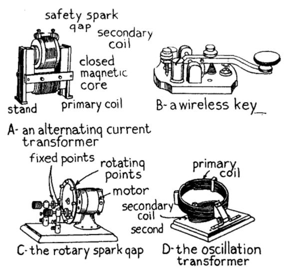
Fig. 21.—Parts for Transmitting Set No. 2.
