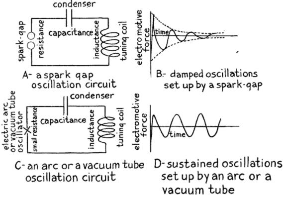
Fig. 35.—Damped and Sustained Electric Oscillations.
