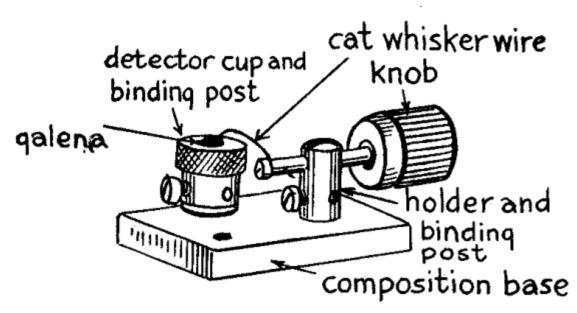
Fig. 96.—Rasco Baby Crystal Detector.
