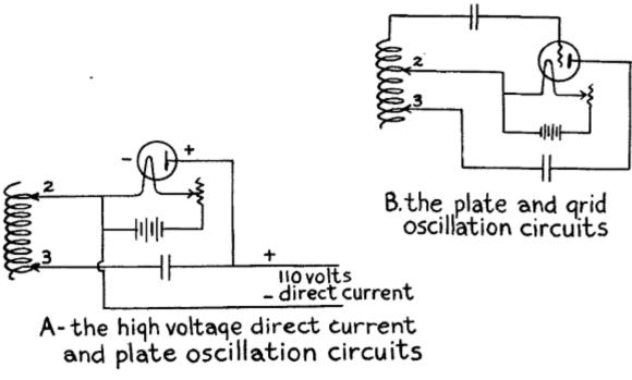
(A) and (B) Fig. 94.—Operation of Vacuum Tube Oscillators.
