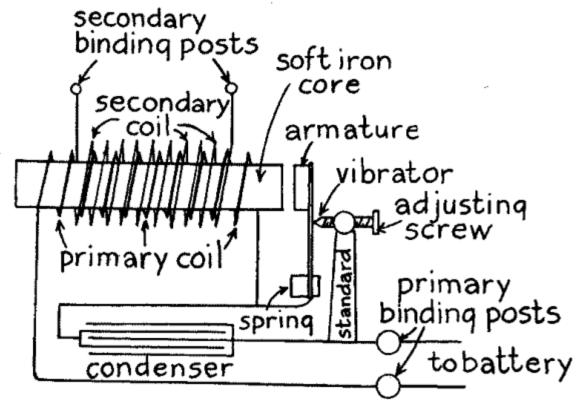
(C) Fig. 18.-Wiring Diagram of Spark Coil.
