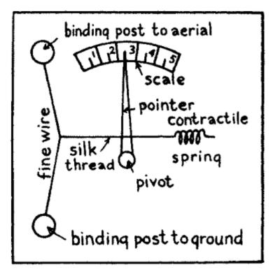
Fig. 24.—Principle of the Hot Wire Ammeter.
