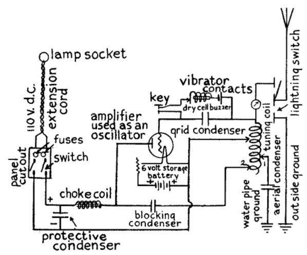
Fig. 76.—Experimental C. W. Telegraph Transmitter.
