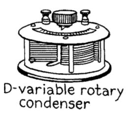
(C) and (D) Fig. 13.—The Variable Rotary Condenser.
