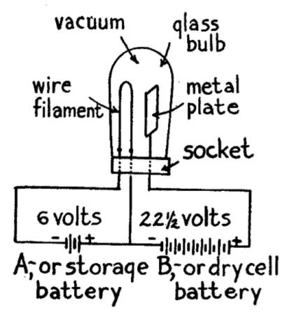
Fig. 37.—Two Electrode Vacuum Tube Detectors.
