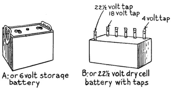
Fig. 39.—A and B Batteries for Vacuum Tube Detectors.
