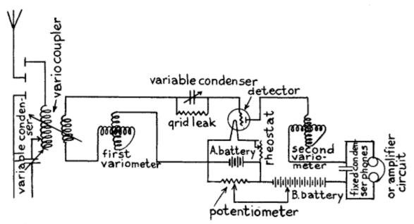
Fig. 56.—Short Wave Regenerative Receiving Set (two Variometer and two Variable Condensers.)
