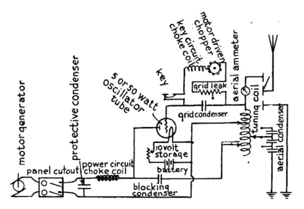
Fig. 78.—5 to 50 Watt C. W. Telegraph Transmitter. (With Single Oscillation Tube.)
