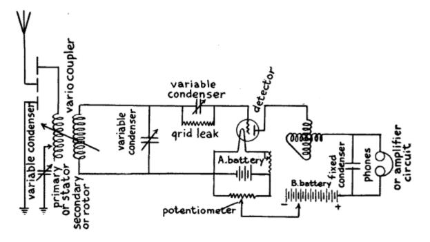
Fig. 55.—Short Wave Regenerative Receiving Set (one Variometer and three Variable Condensers.)
