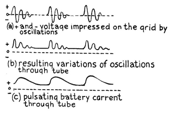
(D) Fig. 72.—How the Oscillations Control the Flow of the Battery Current through the Tube.
