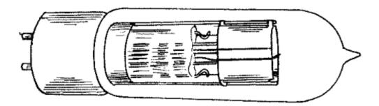
Fig. 80.—50 Watt Oscillator Vacuum Tube.
