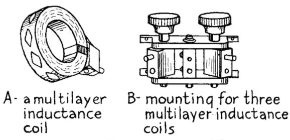
Fig. 50.—Honeycomb Inductance Coil.
