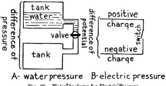
Fig. 28.—Water Analogue for Electric Pressure.
