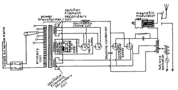
Fig. 93.—100 to 200 Mile Wireless Telephone Transmitter.
