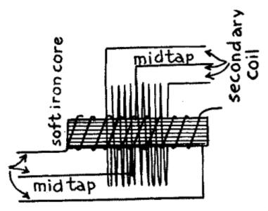
A. wiring diagram of microphone transformer
