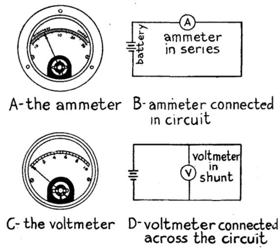
Fig. 30.—How the Ammeter and Voltmeter are Used.
