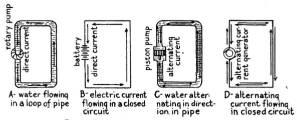
Fig. 29.—Water Analogues for Direct and Alternating Currents.
