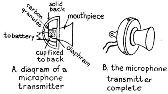
Fig. 84.—Standard Microphone Transmitter.
