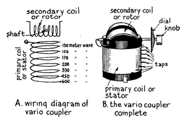
Fig. 53.—How the Variocoupler is Made and Works.
