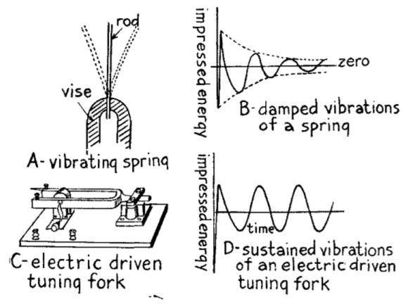
Fig. 34.—Damped and Sustained Mechanical Vibrations.
