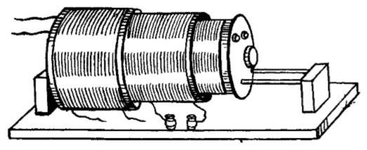
(B) Fig. 49.—Three Coil Loose Coupler Tuner.
