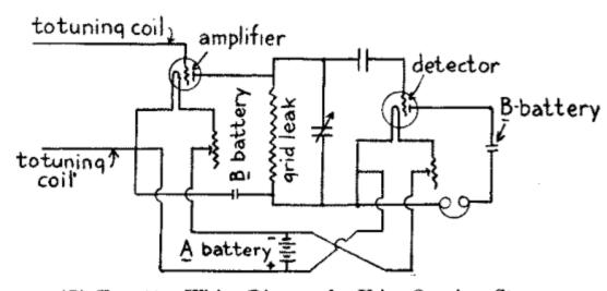
(B) Fig. 44.—Wiring Diagram for Using One A or Storage Battery with an Amplifier and a Detector Tube.
