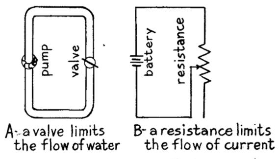
Fig. 31.—Water Valve Analogue of Electric Resistance.
