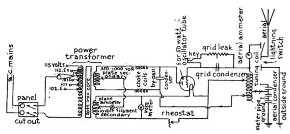
Fig. 82.—Wiring Diagram for 200 to 500 Mile C. W. Telegraph Transmitting Set. (With Alternating Current.)
