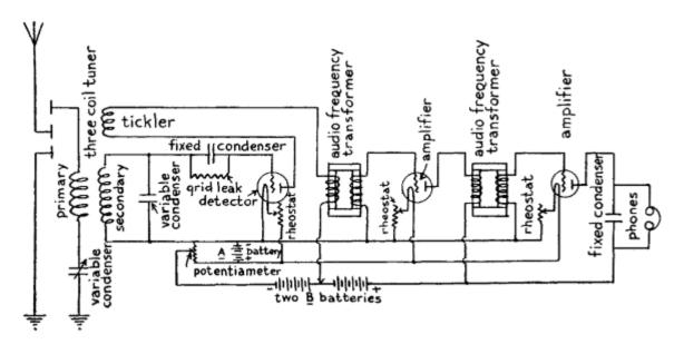
Fig. 52.—Regenerative Audio Frequency Amplifier Receiving Set.
