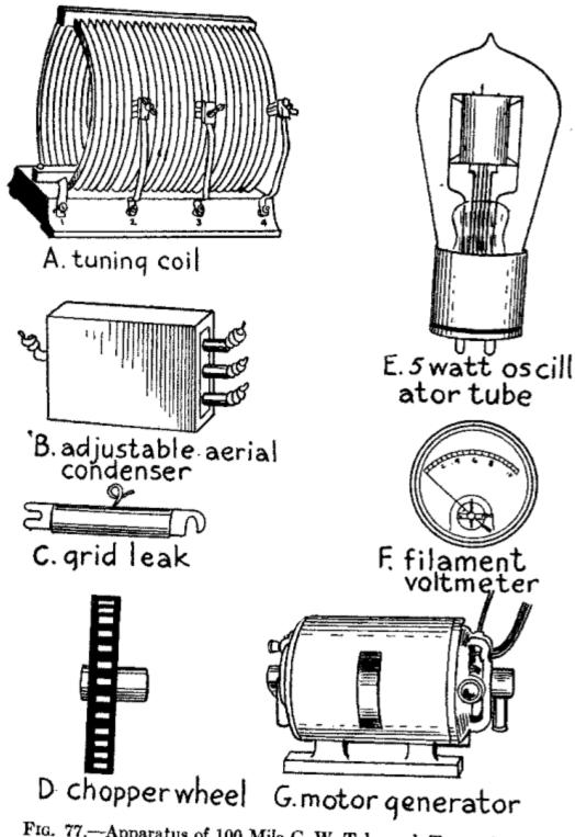
Fig. 77.—Apparatus of 100 Mile C. W. Telegraph Transmitter.
