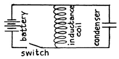
(C) Fig. 94.—How a Direct Current Sets up Oscillations.
