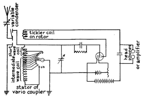
Fig. 58.—Wiring Diagram for Intermediate Wave Receptor with one Variocoupler and 12 section Bank-wound Inductance Coil.
