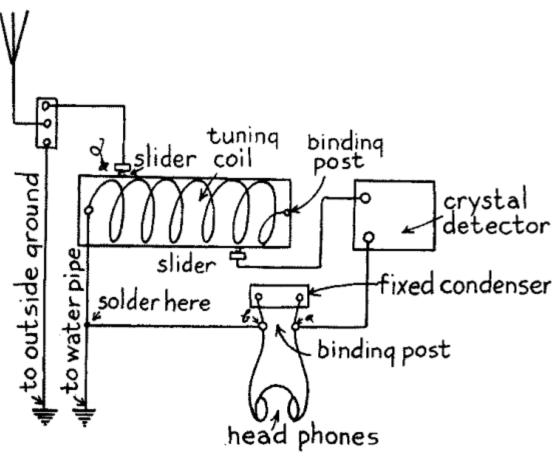
(A) Fig. 15.—Top View of Apparatus Layout for Receiving Set No. 1.
