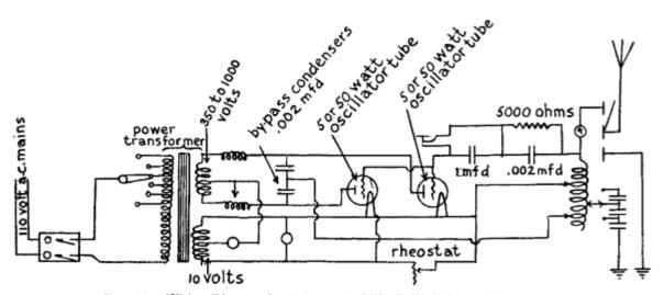
Fig. 83.—Wiring Diagram for 500 to 1000 Mile C. W. Telegraph Transmitter.
