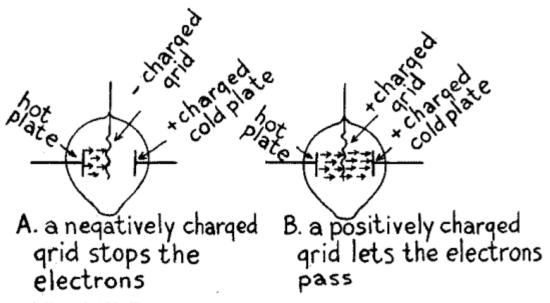
(A) and (B) Fig. 72.—How the Positive and Negative Voltages of Oscillations Act on the Electrons.
