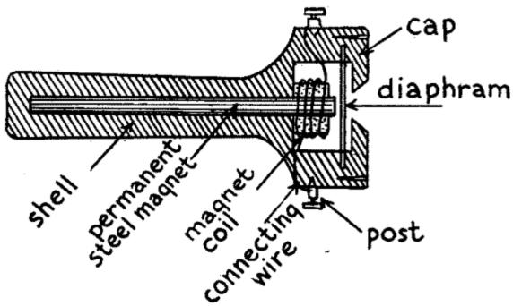
Fig. 62.—Cross-section of Bell Telephone Receiver.
