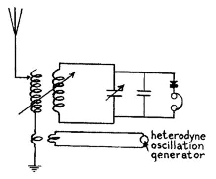
Fig. 74.—Separate Heterodyne Oscillator.
