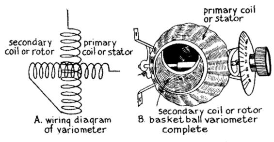
Fig. 54.—How the Variometer is Made and Works.
