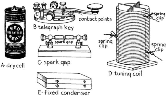
Fig. 19.—Other parts for Transmitting Set No. 1
