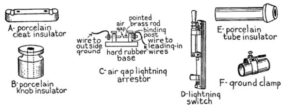
Fig. 5.—Material for a Simple Aerial Wire System.
