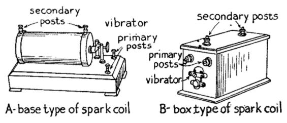
(A) and (B) Fig. 18.—Types of Spark Coils for Set. No. 1.
